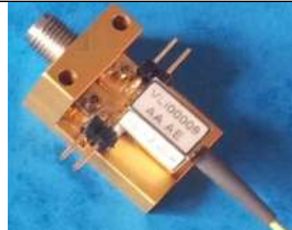
Optical Receiver with coplanar PIN
